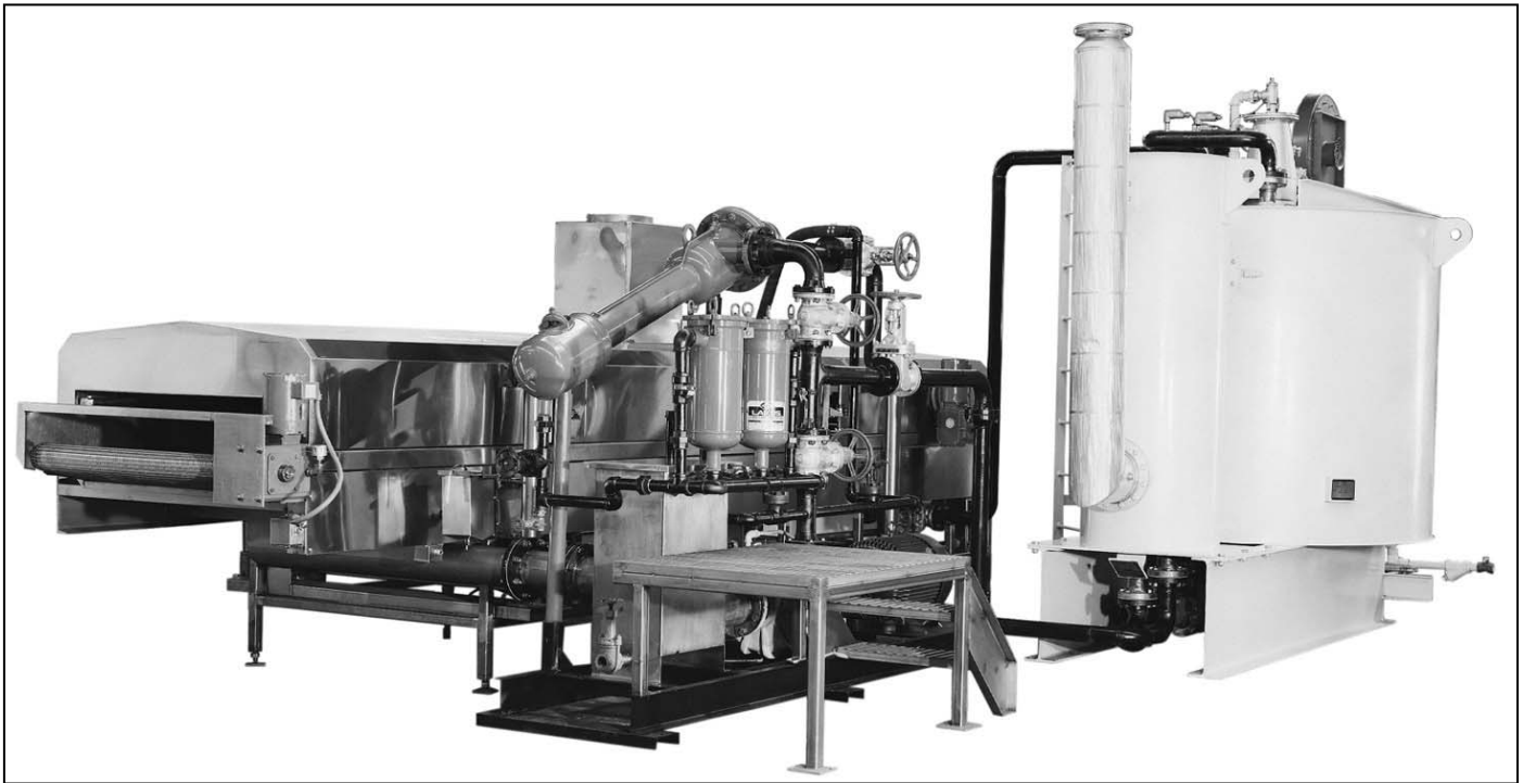
1.75 MM BTU/HR Uniflux vegetable oil heater with a tortilla chip fryer
